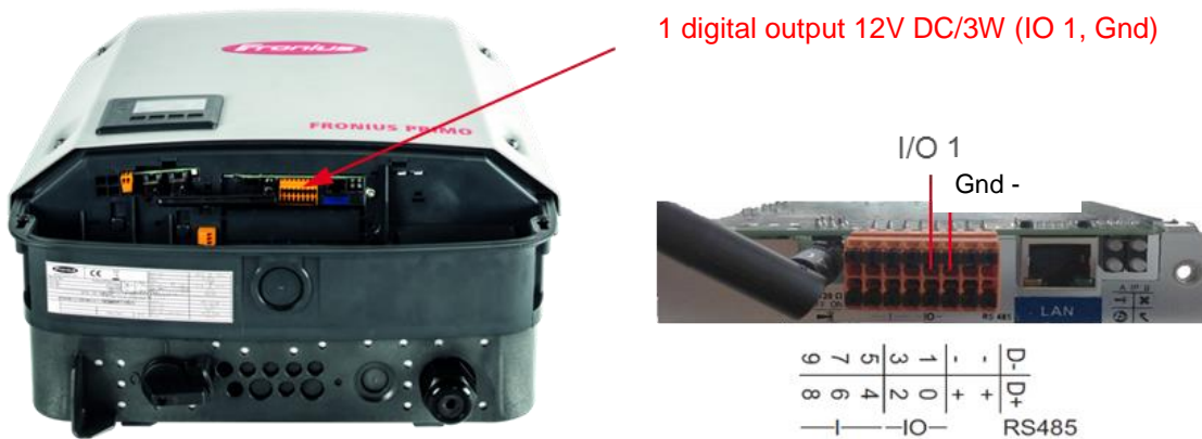
Figure5: Connection on the Fronius Datamanager 2.0 for energy management.
